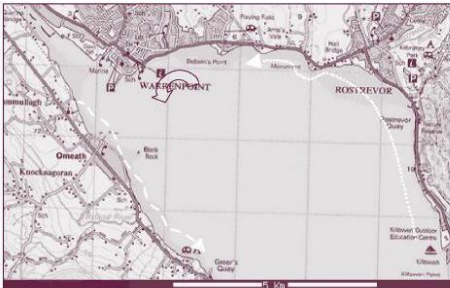
Figure 4.0 A diagrammatical representation of the flushing pattern in Carlingford Lough. (Key: ●●●●●● = tide - - - - = tide out). Map adapted from Northern Ireland Neighbourhood Information Service (2006)
